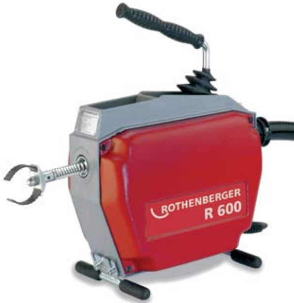
Drive lever locked in stop position — serves as carrying handle
